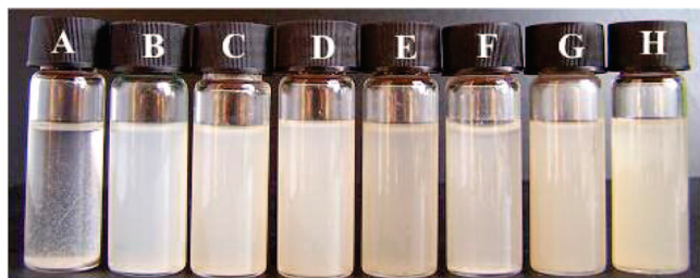
Figure 8. Photos of dispersion status of NDs in different solvents (ca. 1 mg/mL for all samples): (A) pristine ND precipitation in THF, (B) PtBMA-g-ND-g-PS in THF, (C) PtBMA-g-ND-g-PS in DMF, (D) PtBMA-g-ND-g-PS in CHCl 3 , (E) PtBMA-g-ND-g-PS in toluene, (F) PMAA-g-ND-g-PS in water, (G) PMAA-g-ND-g-PS in CHCl 3 , and (H) PMAA-g-ND-g-PS in toluene.
